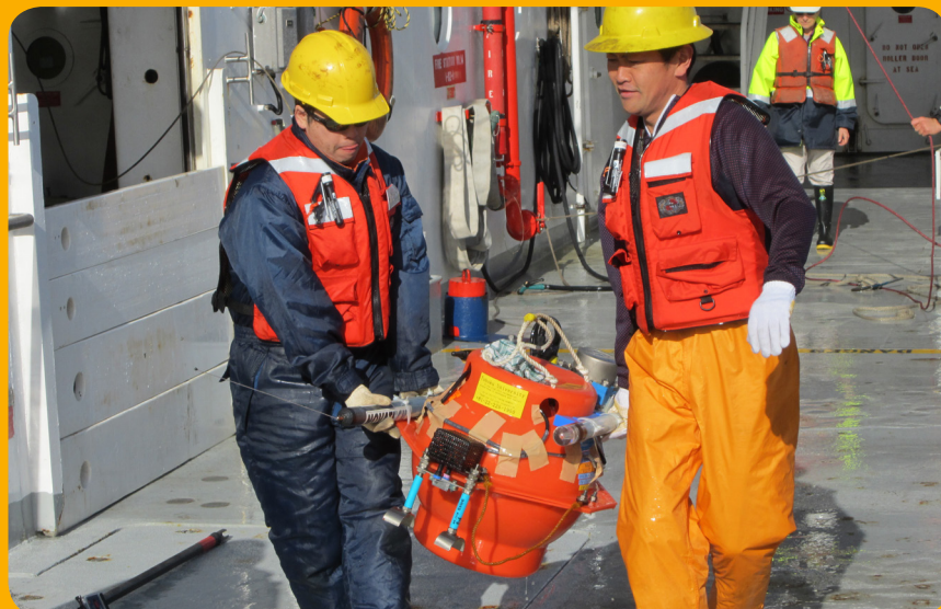
Scientists Kimihiro Mochizuki (Earthquake Research Institute, University of Tokyo) and Syuichi Suzuki (Tohoku University) carry an absolute pressure gauge that recorded over a year's worth of fluctuations in water pressure on the seafloor offshore Gisborne, New Zealand.
